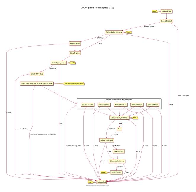
Fig. 2: DHCPv4 packet processing
